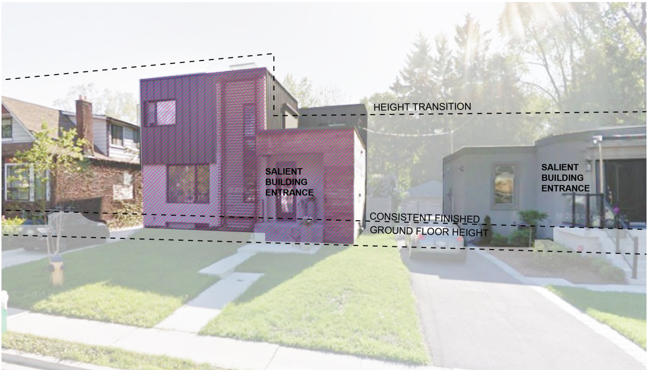
Figure 23: Height and massing transition between existing low-rise buildings
